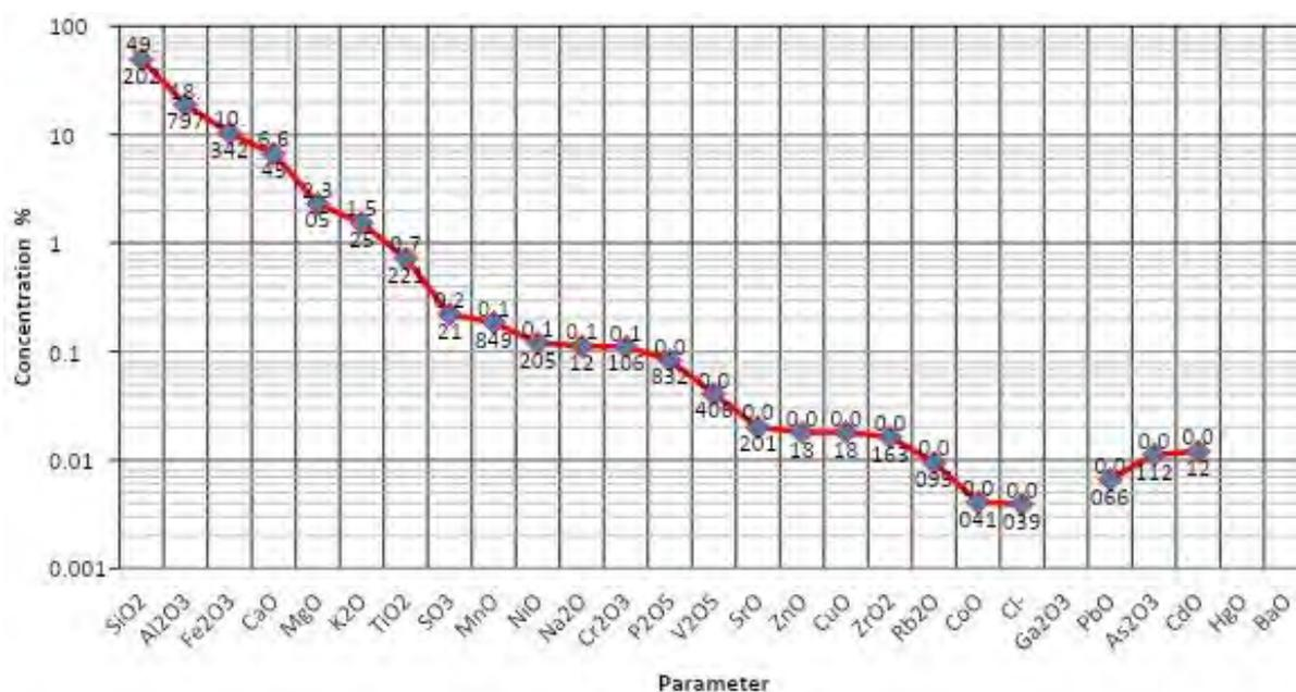
**Figure 3.2.** Chemical composition of slag and ash at Divkovići 2 - Tuzla power plant ash disposal site<sup>10</sup>
