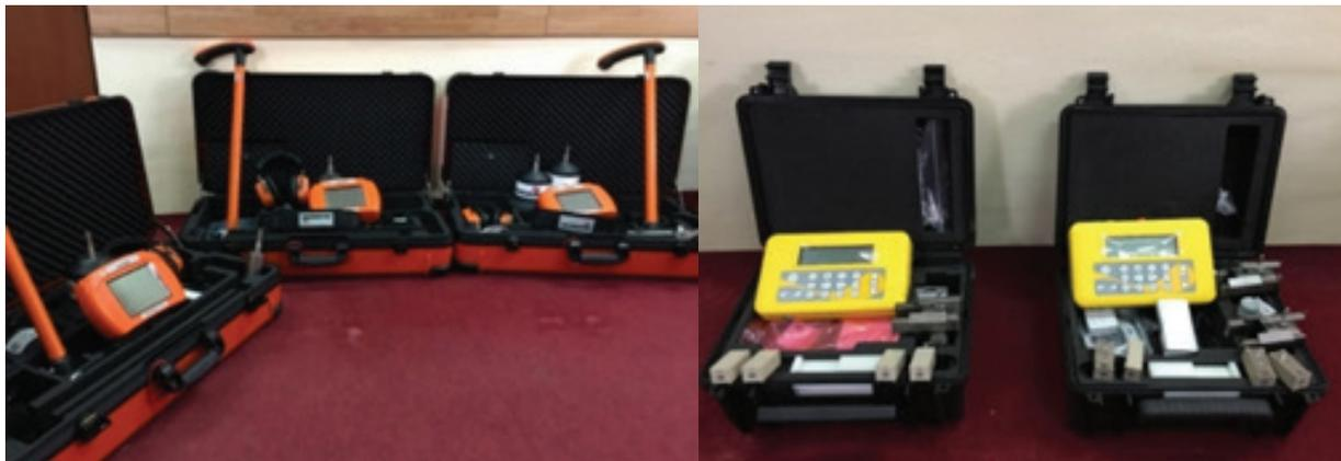
Figure 4.12. Severin A200 water leak detector and Micronis PF 330 portable ultrasonic flow meter
