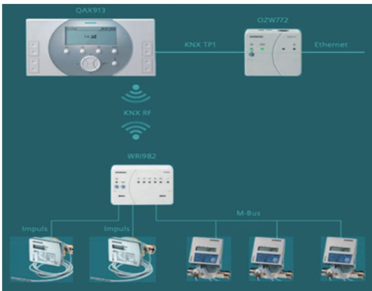
Figure 4.41. An example of a system for monitoring energy consumption [Siemens]
