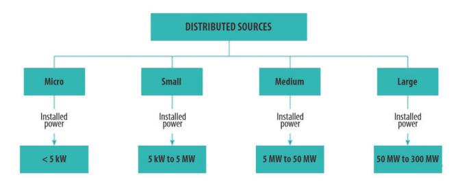
Figure 4.22. Classification of distributed sources according to installed power
