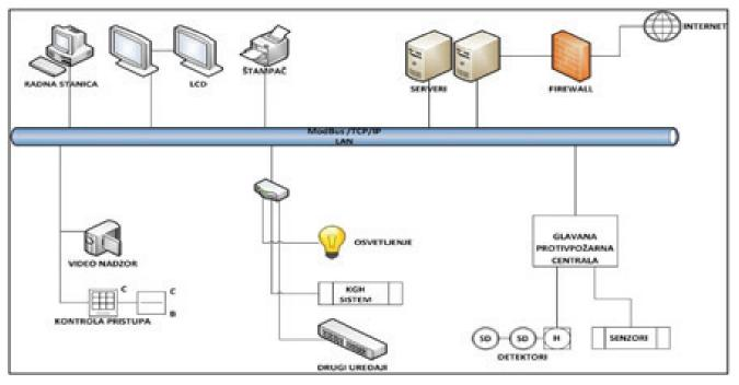
Figure 4.42. Communication links between BMS components
