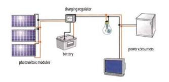
Figure 4.28. Independent PV system with direct current consumers [20]
