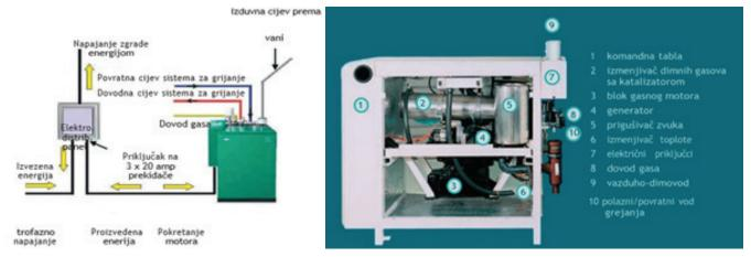
Figure 4.36. a) Micro CHP home system; b) Schematic representation of the ecoPOWER unit
