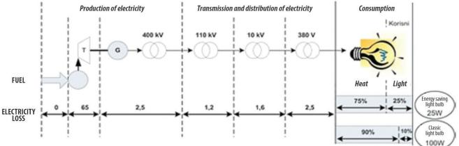
Figure 4.38. Electricity losses on the way to consumption and comparison of two types of light bulbs.
