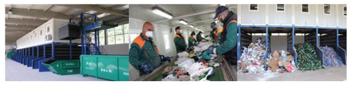
Figure 4.20. Separation of waste into secondary raw materials in the Center for secondary waste selection
