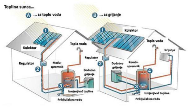
Figure 4.26. The principle of using solar energy for heating sanitary water and rooms
