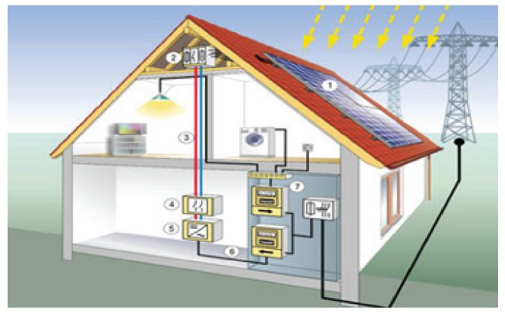
Figure 4.29. Components of a PV system connected to the distribution network: 1- PV panels, 2- charging regulator, 3 – direct current lines, 4 – fuses, 5 – DC/AC inverter, 6 – meter of energy supplied to the network, 7 – meter of energy taken from the network [20]
