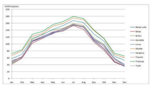
Figure 4.31. Possibilities of production of electric PV panels of 1kW for different cities in Bosnia and Herzegovina [23]
