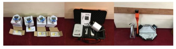
Figure 4.13. Digital pressure gauge DM01, pipe positioning device CG 50 and pipe and cable positioning device Tili Trac R 130
