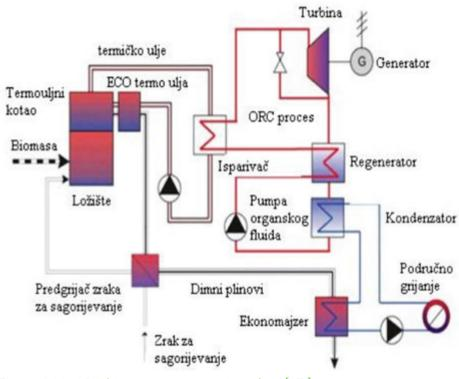
Figure 4.33. ORC biomass cogeneration plant [27]
