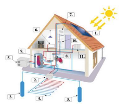
Figure 4.34. Heating and cooling with heat pumps and solar collectors [28]
